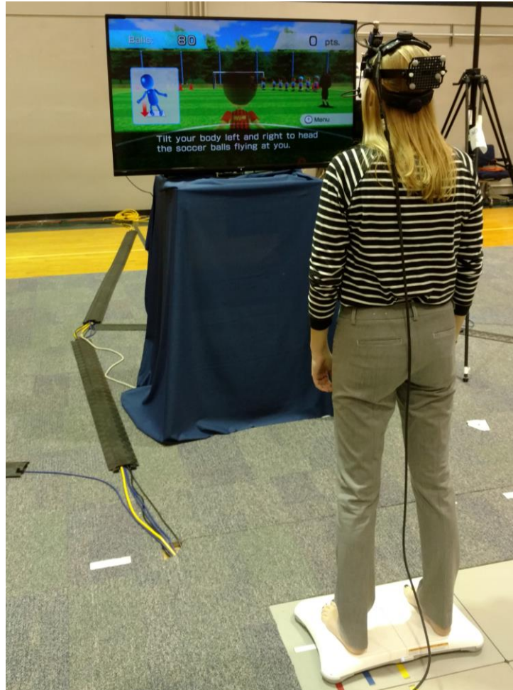
Figure 1. Dynamic, Environmentally-Relevant Postural Assessment: 60-second assessment of the participant playing the WiiFit Soccer Heading game while wearing the ASL Eye Tracker, which sampled the anti-saccade data at a frequency of 240 Hz.
