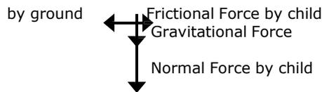
**Figure 1.** Free Body Diagram of a sled
